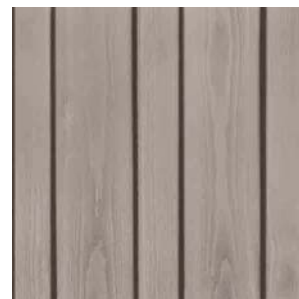
White Fir External cladding
